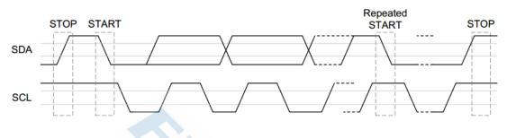
Figure 5: I2C Bus Timing
