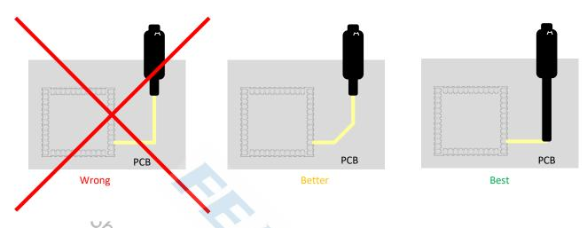
**Figure 12:** Recommended Trace Connects Antenna and the Module
