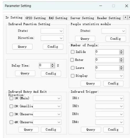
"Ir Setting" label mainly include triggering functions and entry and exit direction judgment functions, etc.
